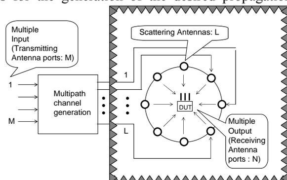
Fig. 1 General configuration of Fading-emulator type MIMO-OTA
