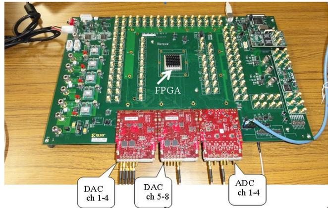
Fig. 6 FPGA installation of Part-1 and -2 of Fig. 3.
