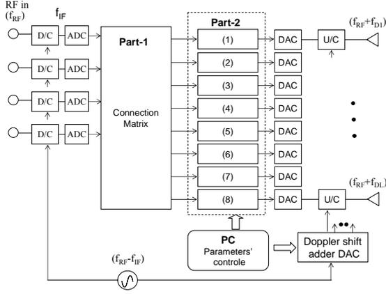
Fig. 3 Basic configuration of the proposed system
