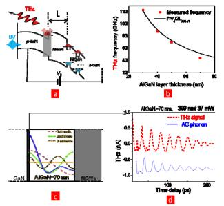
FIGURE 1.(a) Energy band diagram of the sample used in this work. (b) Relation between THz frequency and AlGaN layer thickness. (c) Acoustic standing modes in AlGaN layer. (d) temporal Α comparison between measured THz signal and a simulated acoustic phonon oscillation.
