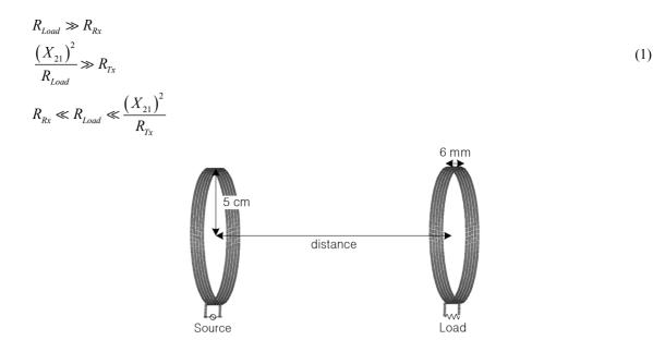
Figure 1: Helix type loop antenna (radius = 5 cm, height = 6 mm, wire thickness = 1 mm, 5 turns, forced resonant frequency = 12.3 MHz).
