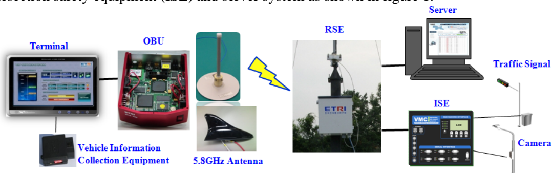
Figure 1: WAVE based vehicular communication system
