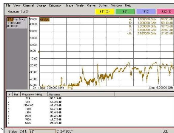
Figure 5. Passive isolation between DSRC and XM antennas.
