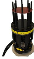
Fig. 1. 8-elements uniform circular array antenna was used at the TX/RX
