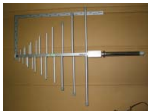
Fig. 4 Picture of the LPDA. The L-angled scale is 50 cm x 25 cm long.
