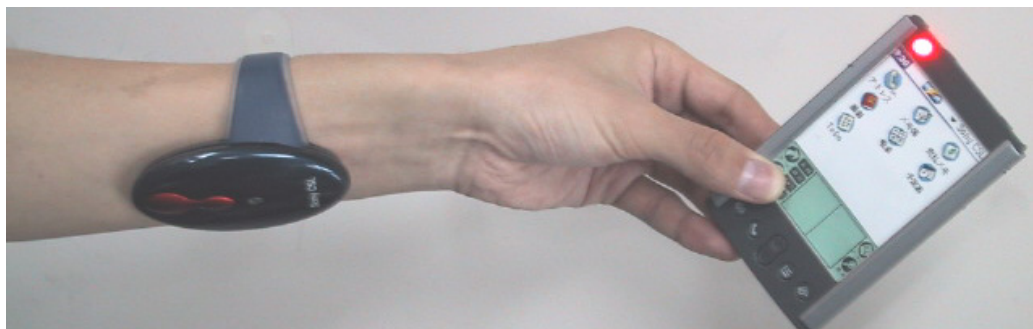
Fig. 1 Transmission system using human body.
