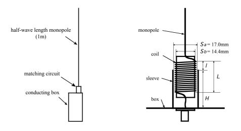
Figure 1. Configuration of the propose antenna.
