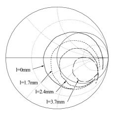
Figure 4. Measured input impedance.
