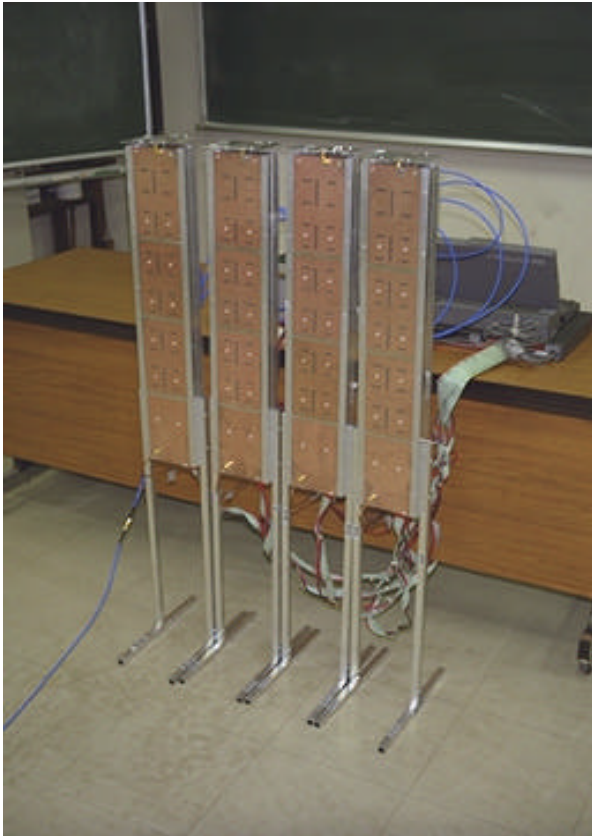
Fig. 3 Picture of the active phased array antenna with the retrodirective antenna system
