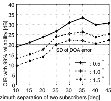
Figure 4: The effect of the direction difference of two subscribers on CIR
