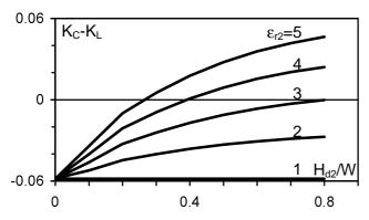
Fig.2. Dependence of difference of capacitive and inductive couplings ( $K_C$ - $K_L$ ) of two coupled microstrip lines with covering dielectric layer on height of the layer  $H_{d2}/W$  for various relative permittivities of the layer  $\epsilon_{r2}$ =1-5.  $H_{d1}/W$ =0.5,  $\epsilon_{r1}$ =3, D/W=3, S/W=1.
