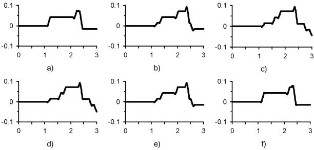
Fig.5. Waveforms (V, ns) of far-end crosstalk when increasing the position ( $\ell_1$ =0,2...10 cm, plots a-f, accordingly) of the section with covering dielectric layer.
