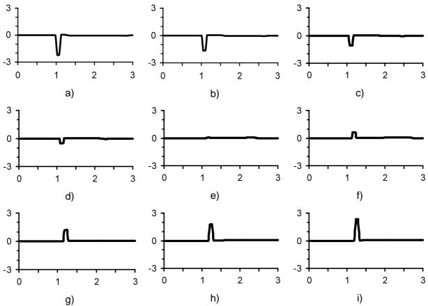
Fig.4. Far-end crosstalk waveforms (V, ns) calculated for increasing length ( $\ell_2$ =2,4...18 cm) of the section with covering dielectric layer, while  $\ell_1$ =0 and  $\ell_2$ + $\ell_3$ =20 cm (plots a-i, accordingly).
