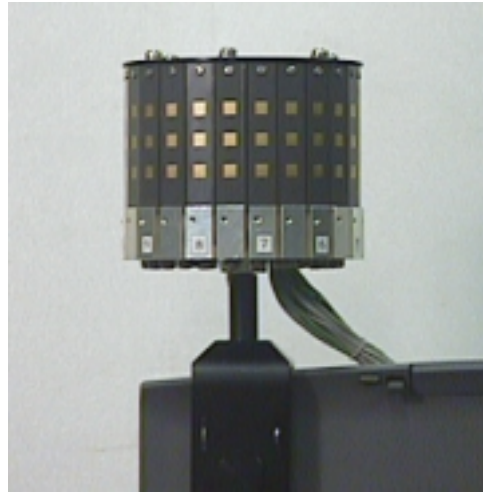
Photo. 1 Photograph of prototype cylindrical 12-sector antenna
