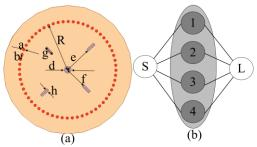
Fig. 1. Circular SIW cavity resonator configuration.
