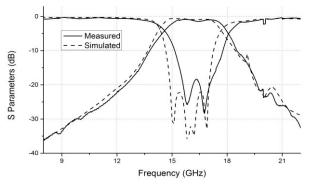
Fig. 5. Simulated and measured S parameters of the filter.
