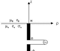
Figure 2: The model of underground asymmetric dipole antenna
