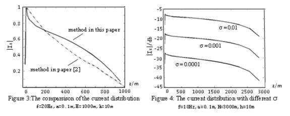
In this paper, the underground asymmetric dipole antenna current integral equation is deduced to avoid the SI calculus, which greatly simplifies the theoretical analysis and computational complexity and better meet the needs of practical engineering. This is a method of great engineering value.
