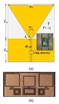
Fig. 2. (a) Geometry of the sensing antenna with chip detector; (b) chip photo of the liquid detector [1].
