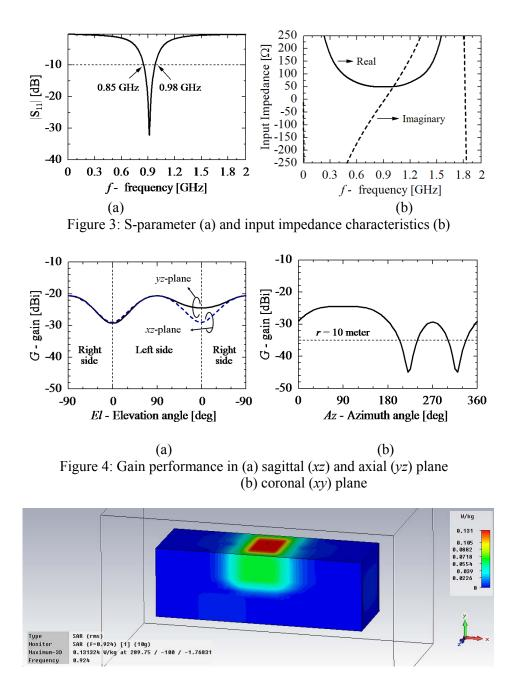
Figure 5: Result of 10g-averaged SAR calculation at 924 MHz
