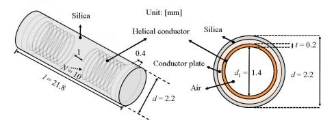
Figure 1: Antenna structure
