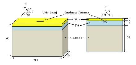
Figure 2: Antenna in tissue structure
