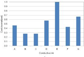
Fig. 6. Cost of 1 mm<sup>3</sup> conductive inks.
