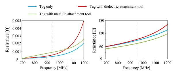
Figure 6: Impedance of RFID tag antenna.
