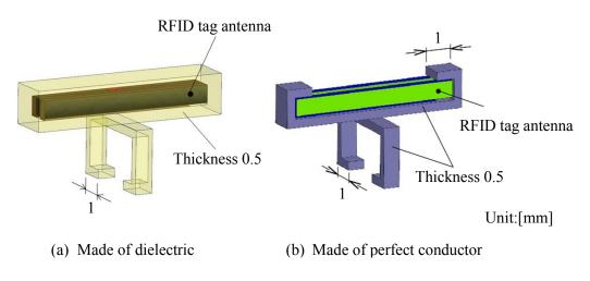
Figure 3: Structure of the RFID tag antenna attachment tools.
