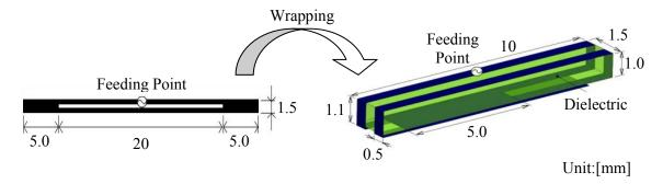
Figure 1: Structure of the proposed tag antenna.
