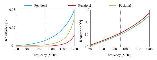
Figure 4: Impedance of RFID tag antenna.
