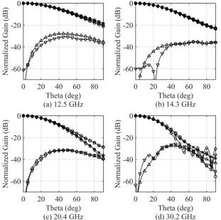
Fig. 3 Comparison of radiation patterns by MMM and CST at the center frequency of each band (MMM 0°-plane co-pol -□-, CST 0°-plane co-pol -○-, MMM 90°-plane co-pol -\*-, CST 90°-plane co-pol -◇-, MMM 45°-plane cross-pol -△-, CST 45°-plane cross-pol -▽-)
