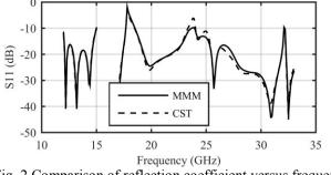
Fig. 2 Comparison of reflection coefficient versus frequency by MMM and CST
