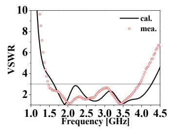
Figure 6: VSWR characteristics of proposed antenna
