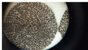
Fig. 3. Full-embroidered Model: Close up photo of the half side of the radiating element.
