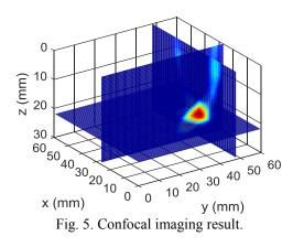
Finally, the confocal imaging algorithm is applied to the subtracted signals to recognize the position of the target [1]. Figure 5 shows the confocal imaging result. The estimated position is x=27, y=48, z=22 mm, compared with the actual position x=28, y=46, z=26 mm.
