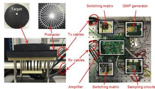
Fig. 1. Experiment setup and breast phantom.
