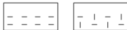
(b) Horizontal polarization (c) Multi polarization Figure 1. Imaging sensor with various polarizations
