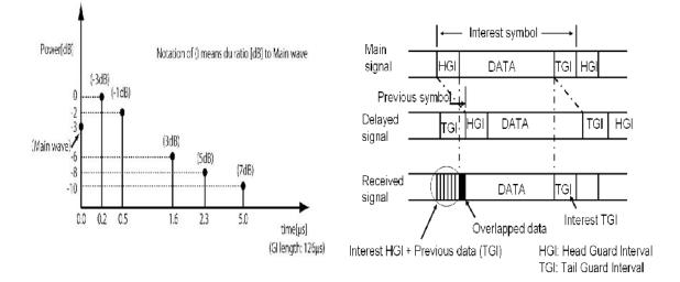
Figure 2: Delay Spread Profile
