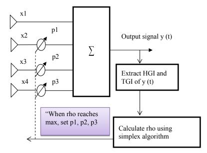
Figure 1:Block Diagram of Proposed Diversity Antenna
