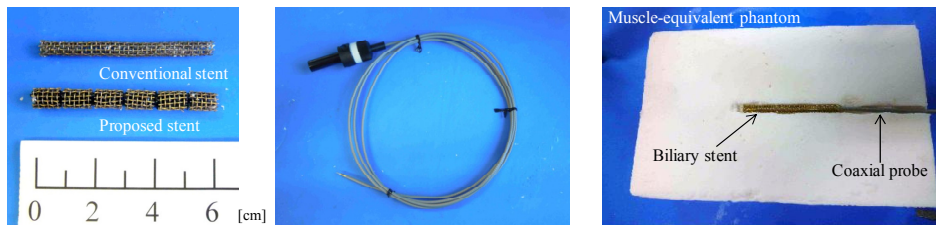
(a) Trial manufactures of stents. (b) Endoscopic probe. (c) Setup.
