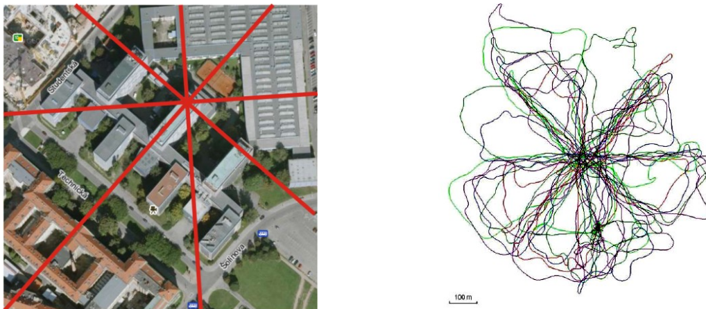
Figure 2: Flyovers of the airship above a selected building (left), five actual flight paths above building A including airship manoeuvres (right)
