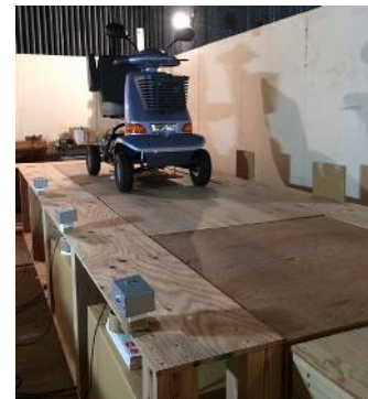
Fig. 2 WPT system for traveling mobility scooter.
