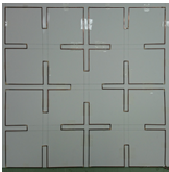
Fig.4 Fractal loop and matching circuit
