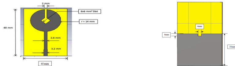
Figure 1: Proposed Antenna (Front and Back View)
