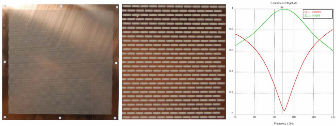
Fig. 2. Photograph of fabricated polarizing grid and its S-parameter
