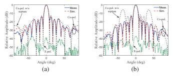
Fig. 6. Simulated and measured radiation patterns of the proposed array antenna at 81 GHz. (a) E-plane, (b) H-plane.
