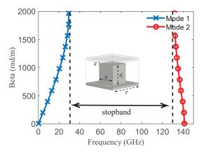
Fig. 2. Dispersion diagram of the infinite periodic pin unit cell  $(d_f = 0.68 \text{ mm}, a = 0.64 \text{ mm}, g = 0.04 \text{ mm}, \text{and } p = 1.28 \text{ mm}).$
