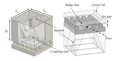
Fig. 1. The proposed horn unit cell ( $L_E=6\ mm,\ L_H=6.1\ mm,$  and  $H=5\ mm)$
