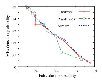
Fig. 6. False alarm probability and miss-detection probability of the proposed methods (5 GHz band).
