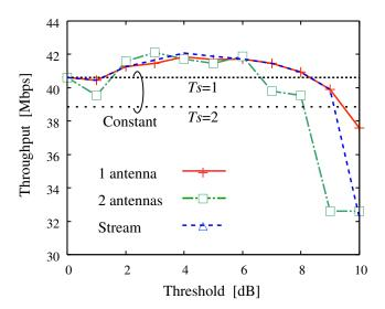
Fig. 7. Throughput as a parameter of threshold (5 GHz band).
