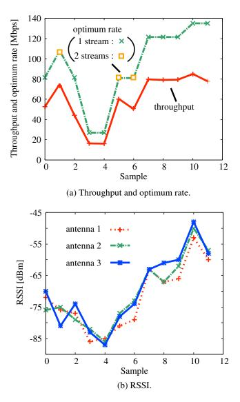
Fig. 5. Example of measurement result at each sample (5 GHz band).
