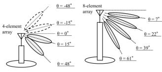
(a) 4-element butler matrix (b) 8-element butler matrix Figure 1. Antenna pattern in vertical pattern
