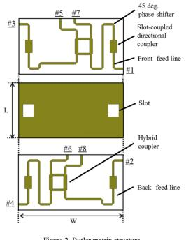
Figure 2. Butler matrix structure L = 84, W=160 [mm]
