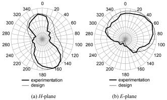
Fig. 5. Radiation patterns of experimentation and design results
