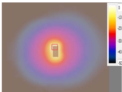
Fig. 4. Simulated 1-g average SAR distribution for the designed antenna.
