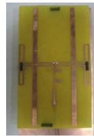
Fig.6. Structure of antenna with low pass filter
