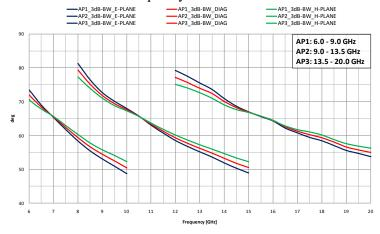
Figure 5: 3dB Beamwidth with frequency (AP1:6-9GHz, AP2: 9-13.5GHz & AP3: 13.5-20GHz).
