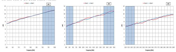
Figure 3: Boresight gain with frequency - (AP1: 6-9GHz, AP2: 9-13.5GHz & AP3: 13.5-20GHz).
