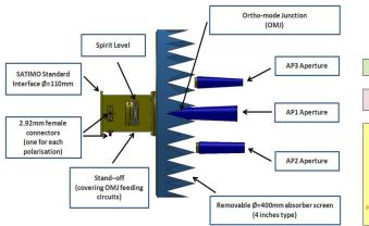
Figure 1: Dual linear polarized probe covering the entire 6GHz to 20GHz frequency bandwidth with three interchangeable apertures (6-9GHz, 9-13.5GHz & 13.5-20GHz.
