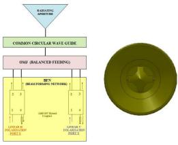
Figure 2: Left - Block diagram of four excitation pin polarizer network for L/Ka-band orthomode junction. Right - Front view of the probe topology showing the inverted quad ridge structure of the probe.
