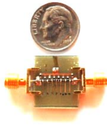
Figure 3. Fabricated 7-section LH NLTL phase shifter using FR4 substrate.
