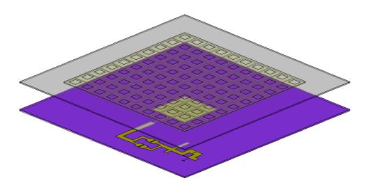
Figure 2 : Layout of the proposed rectenna using the AMC as the superstrate.
