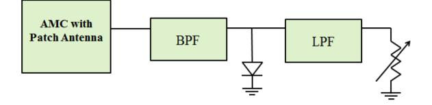
Figure 1 : Block diagram of the rectenna.
