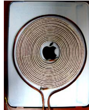
Figure 6: Measured S-parameters. Figure 7: The proposed resonator on the tablet PC.
