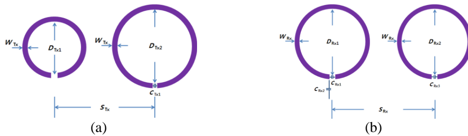
Figure 1: Wireless energy transmission resonator having large circular transmitting and small circular receiving coils (a) Transmitting coil, (b) Receiving coil.
