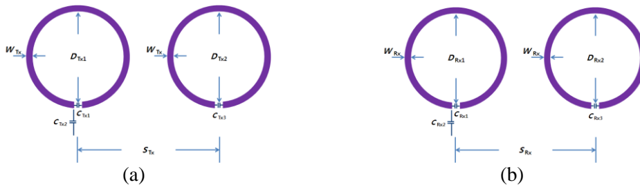
Figure 5: Wireless energy transmission resonators having various-sized circular transmitting and receiving coils (a) Transmitting coil, (b) Receiving coil.
