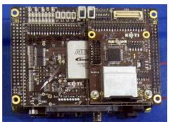
Figure 3: Proposed hardware platform including MOST INIC, SRAM-MLB and EHC based on RISC process
