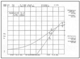
Figure 5: AM-PM characteristics for the linearizer at 8.15GHz
