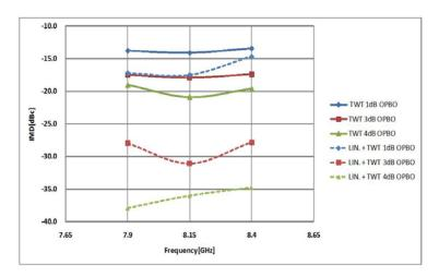
Figure 8: Improved IMD of the TWTA using linearizer
