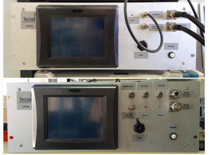
Fig. 3: Channel sounder transmitter and receiver.
