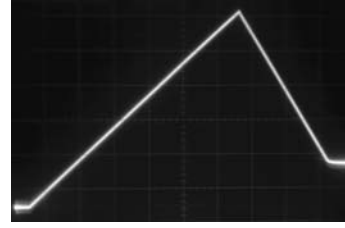
Figure 7: Nonlinear function f(x) . Horizontal axis: x (1V/div); vertical axis: f(x) (1V/div).
