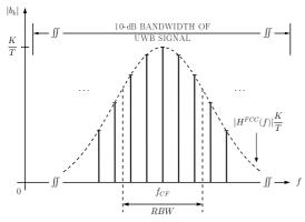
Figure 4: The spectrum of the response of Gaussian filter used in spectrum analyzers, i.e. the FCC filter to the UWB IR carrier train.
