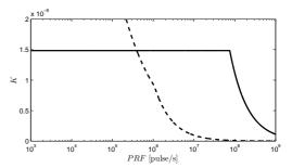
Figure 5: Maximum allowable values of parameter K versus pulse repetition frequency. The solid and dashed curves show the values of parameter K that are compliant to the FCC peak and average, respectively, power limits. The RBW values are 1 MHz and 50 MHz for the FCC peak and average power limits, respectively.
