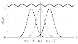
Figure 3: Envelope of FCC filter output when PRF > RBW. Note, the FCC filter outputs generated by the individual UWB pulses overlap one another.
