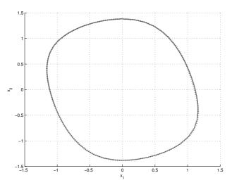
Figure 2: Limit cycle for the Van der Pol oscillator: solid grey line (HB approximation), dotted black line (time-domain simulation).
