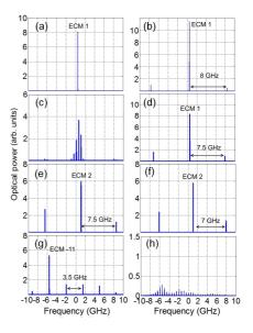
Figure 5: Optical spectrum with the initial condition ECM 1 for (a)  $\eta = 0.15$ , (b) 0.24, (c) 0.35, (d) 0.42, (e) 0.47, (f) 0.55, (g) 0.75, and (h) 0.9.
