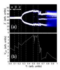
Figure 2: (a) Reverse BD for I = 22.59 mA and L = 30 cm and (b) the corresponding  $V_{\rm LD}$ .
