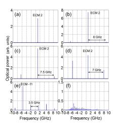
Figure 6: Optical spectrum with the initial condition ECM 2 for (a)  $\eta$  = 0.2, (b) 0.3, (c) 0.39, (d) 0.55, (e) 0.7, and (f) 0.9.
