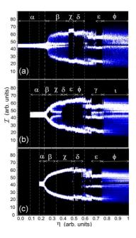
Figure 3: Forward BDs for several initial conditions for I = 22.59 mA and L = 30 cm; Initial mode: (a) ECM 0, (b) ECM 1, and (c) ECM 2.
