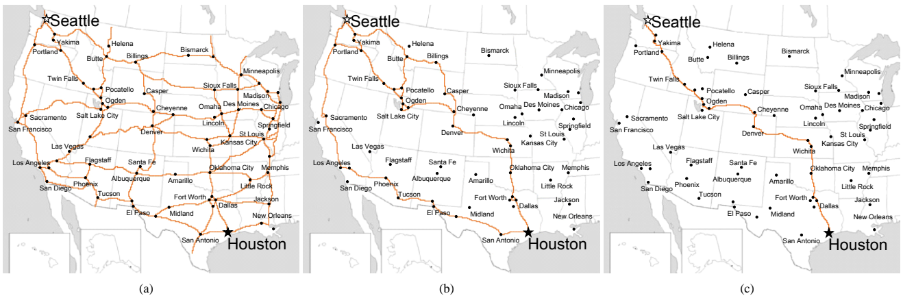
Figure 5: (a) The network of US interstate highway is indicated by the orange lines. The start point (Houston) and the goal (Seattle) are indicated by black and white stars, respectively. (b) All conceivable routes which are obtained by APA. There are not only the shortest path, but also a near routes. (c) The shortest path.
