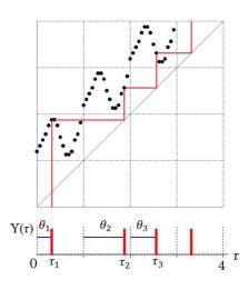
Figure 1: Digital spike-position map and spike-train
